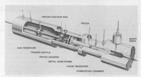
SANDIA-DEVELOPED FIXTURE, called a liquid-propellant injector/combustor, provides critical information about the origin of pressure oscillations observed in liquid-propellant firings of a prototype 155mm howitzer.
